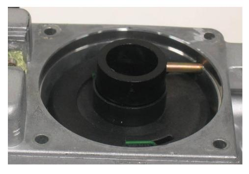
Step 4) Put the new SACER tps sensor cap in place. Make sure the rubber O-ring is correctly in place.
