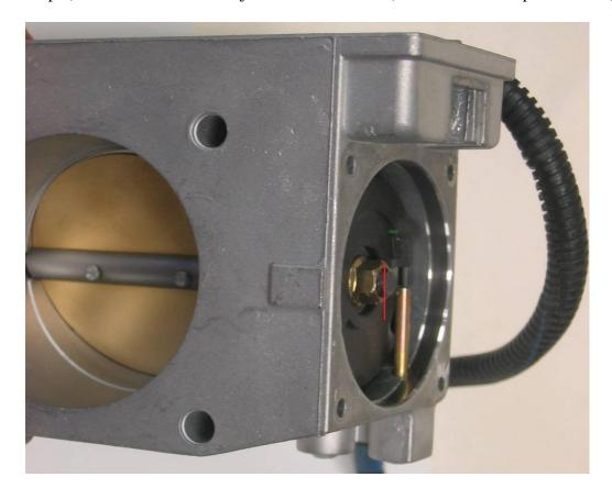
Step 3) Remove the nut, put the magnet on place, and mount the Nut again, adding some LOCTITE!
